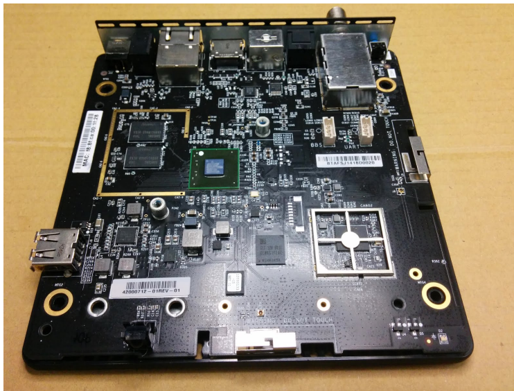
Top of PCBA, heatsink and WLAN RF shield removed:
