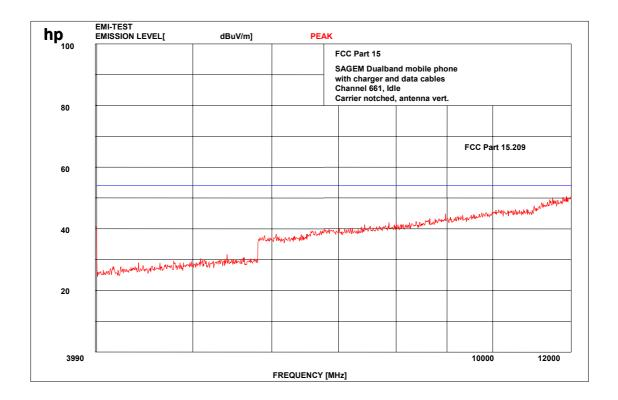
f < 1 GHz : RBW/VBW: 100 kHz f ≥ 1GHz : RBW 1 MHz/VBW: 10 Hz (Average)
