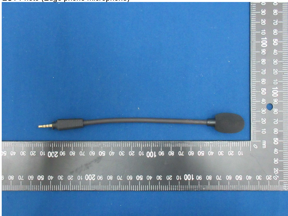
(24) EUT Photo (Edge phone microphone)
