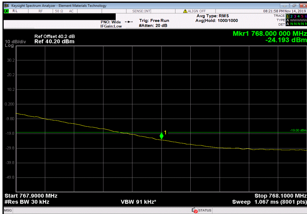
Band 14, QPSK Modulation, LTE5 Bandwidth, Upper Band Edge, Measurement 2
