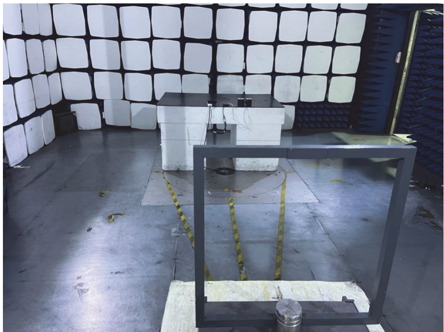
Radiation Emission Test Setup (Below 30MHz)
