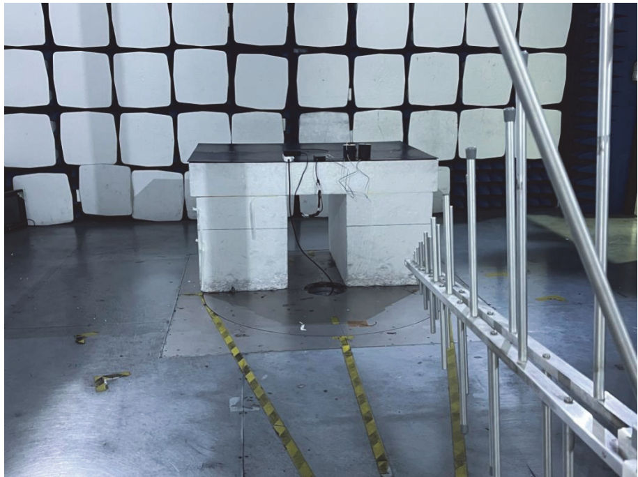
Radiation Emission Test Setup (30MHz to 1GHz)
