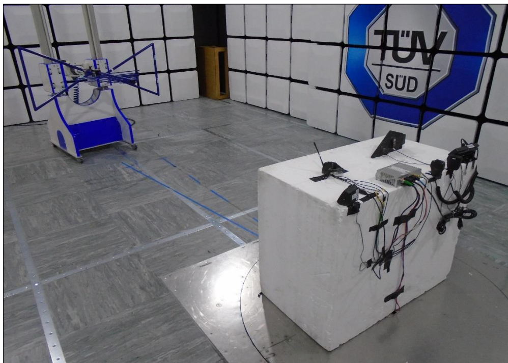
Figure 6 - Test Setup - Below 1 GHz
