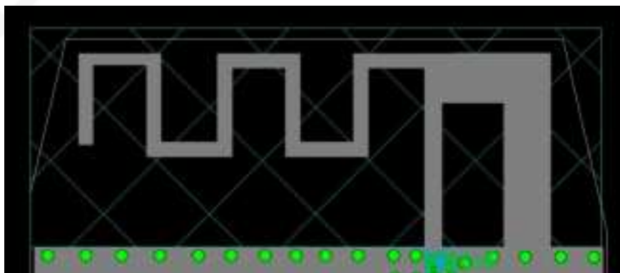
Fig 2 BL1206-P Antenna layout
