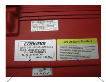
Label with FCC ID:NEODSBR4008PS and IC:8749-DSBR4008PS is located here. The Warning label is located here.
