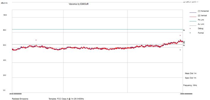
Radiated Emissions Template: FCC Class A @ 1m 20.0-40GHz Filename: c:/program files (x88)/emisoft - vasona/results/Chargepoint 28.5-40GHz eRAT.emi
