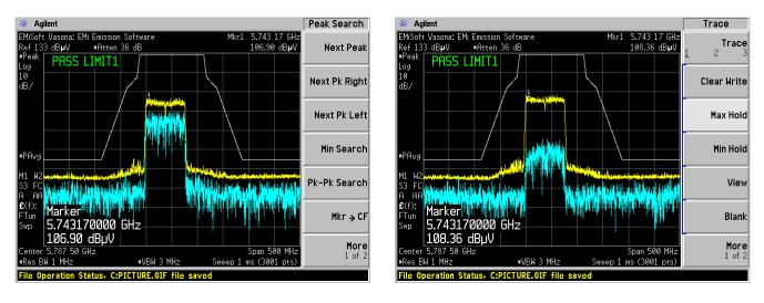
Note: For 5.8 GHz Band Emission Mask measurements, equipment factors were considered into offset on PSA.
