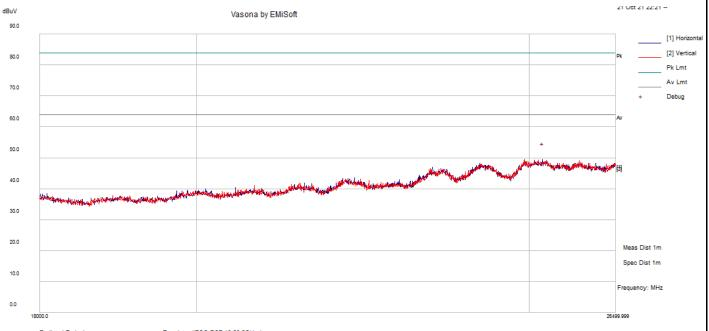
Radiated Emissions Template: #FCC RSE 18-26.5GHz 1m Filename: c:\program files (x88)\emisoft - vasona\results\Chargepoint 18-26.5GHz 5wifi.emi
