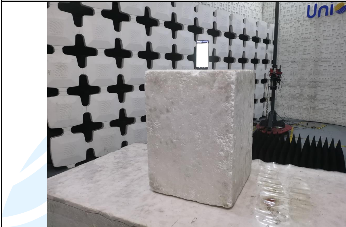
Radiated emission Test Setup (Above 1 GHz)
