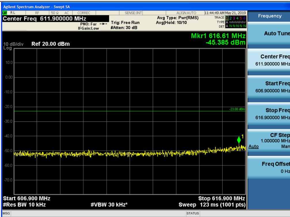
Spurious / 600 MHz Service / Downlink / LTE 10 MHz / High / High Edge + 0.1 MHz ~ High Edge + 10.1 MHz
