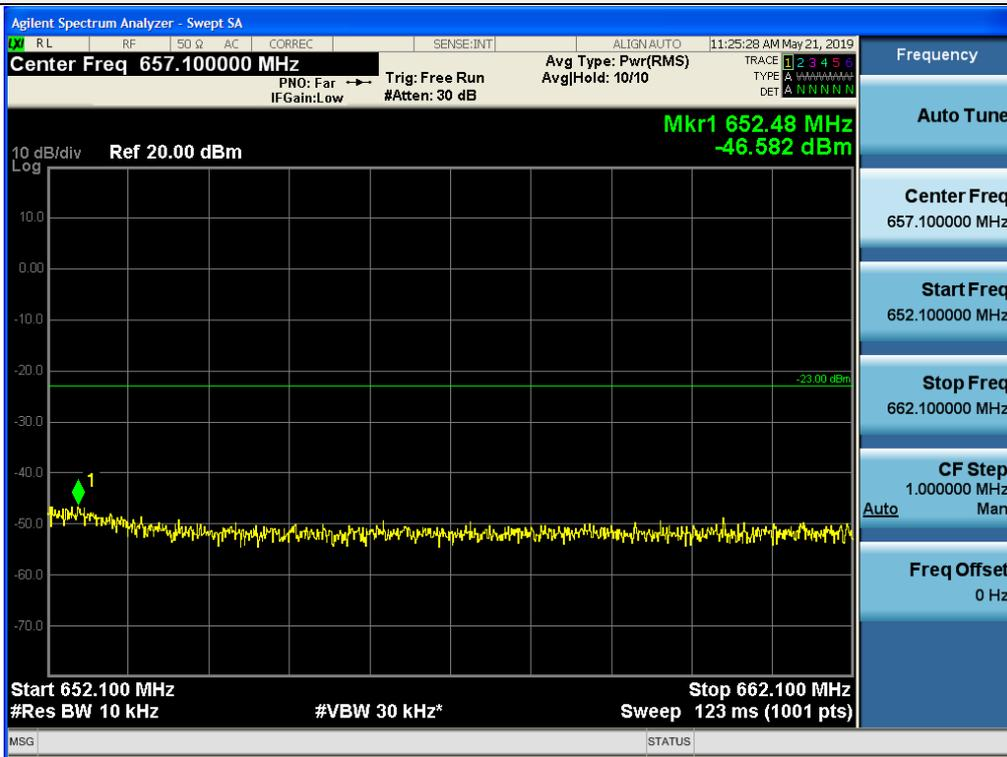
Spurious / 600 MHz Service / Downlink / LTE 20 MHz / Low / High Edge + 10.1 MHz ~ 1 GHz
