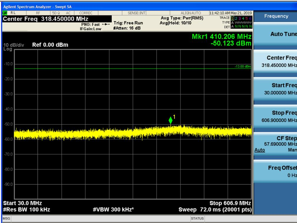
Spurious / 600 MHz Service / Downlink / LTE 10 MHz / Low / Low Edge - 10.1 MHz ~ Low Edge - 0.1 MHz
