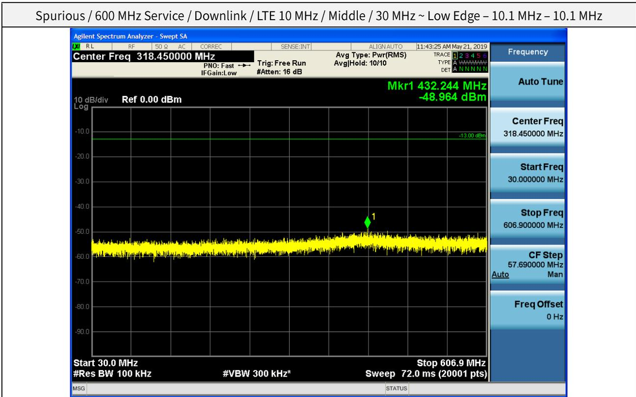
Spurious / 600 MHz Service / Downlink / LTE 10 MHz / Middle / Low Edge - 10.1 MHz ~ Low Edge - 0.1 MHz
