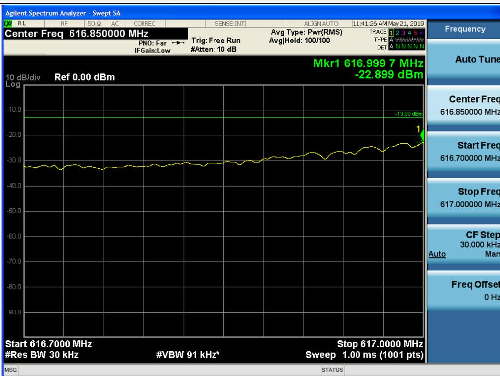
+3 dB above Out-of-band (single test signal) / 600 MHz Service / Downlink / LTE 20 MHz / Upper
