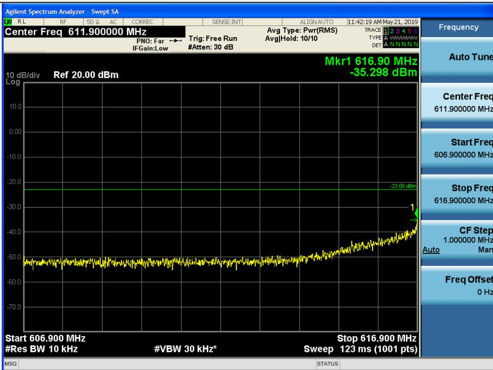
Spurious / 600 MHz Service / Downlink / LTE 10 MHz / Low / High Edge + 0.1 MHz ~ High Edge + 10.1 MHz
