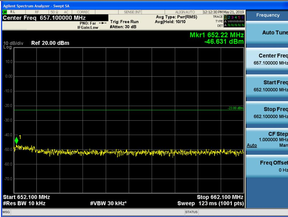
Spurious / 600 MHz Service / Downlink / LTE 5 MHz / Low / High Edge + 10.1 MHz ~ 1 GHz
