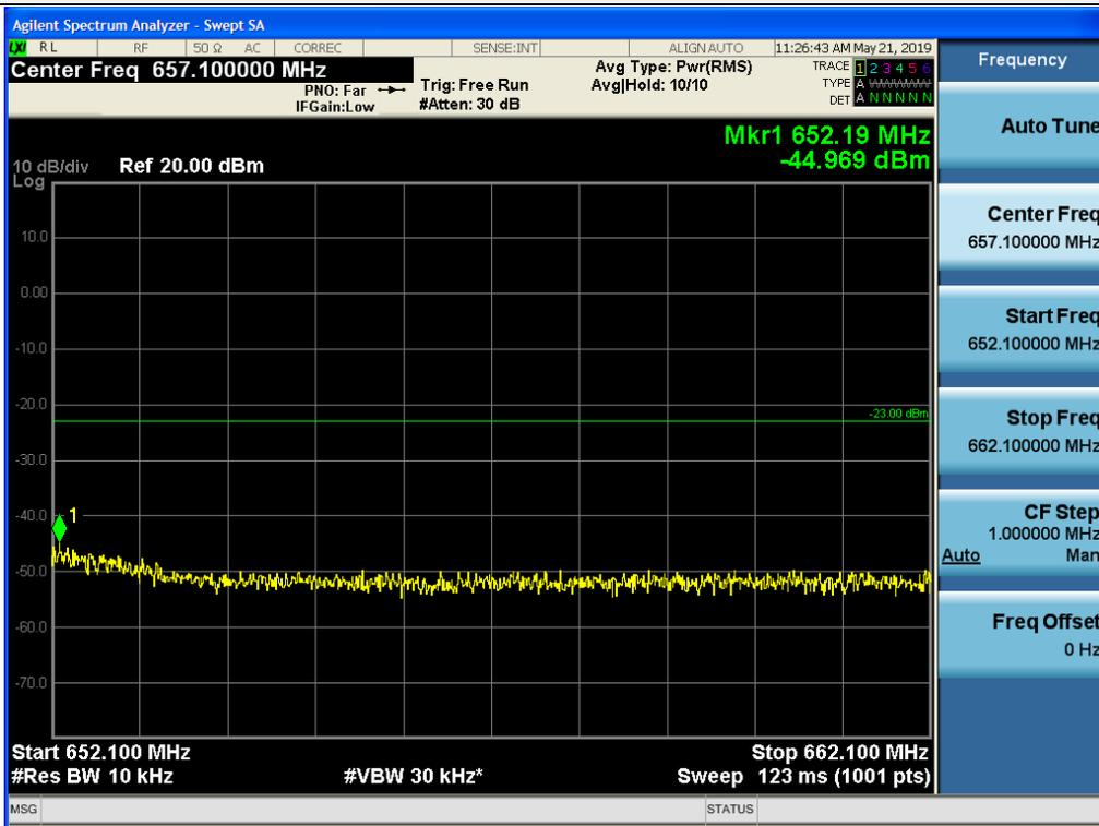
Spurious / 600 MHz Service / Downlink / LTE 20 MHz / Middle / High Edge + 10.1 MHz ~ 1 GHz
