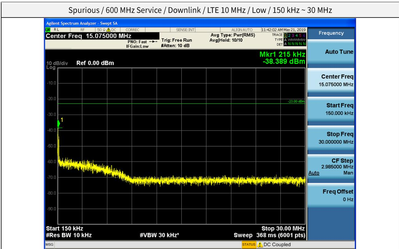
Spurious / 600 MHz Service / Downlink / LTE 10 MHz / Low / 30 MHz ~ Low Edge - 10.1 MHz - 10.1 MHz
