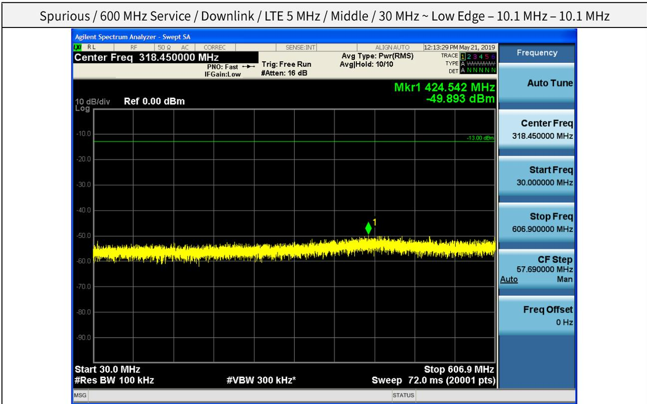
Spurious / 600 MHz Service / Downlink / LTE 5 MHz / Middle / Low Edge - 10.1 MHz ~ Low Edge - 0.1 MHz
