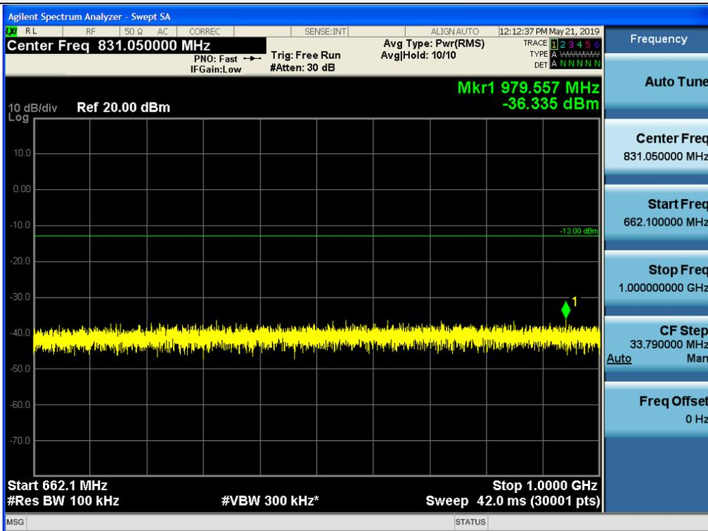
Spurious / 600 MHz Service / Downlink / LTE 5 MHz / Low / 1 GHz ~ 10 GHz
