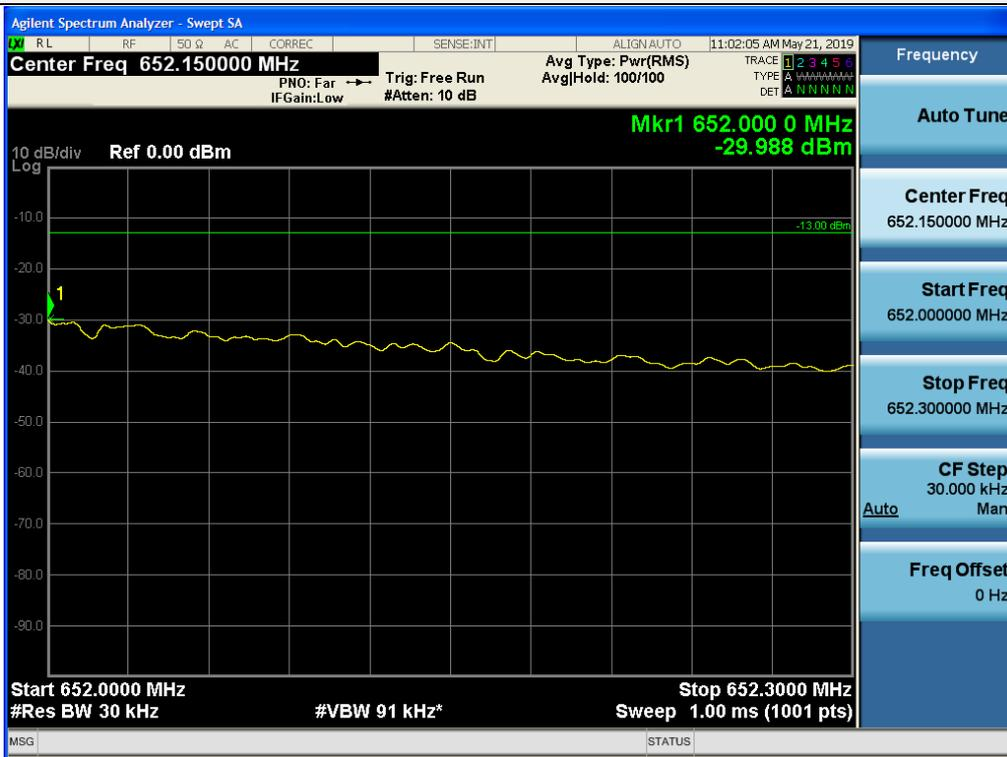
Out-of-band (single test signal) / 600 MHz Service / Downlink / LTE 20 MHz / Lower
