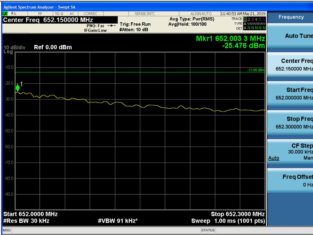
+3 dB above Out-of-band (single test signal) / 600 MHz Service / Downlink / LTE 10 MHz / Lower
