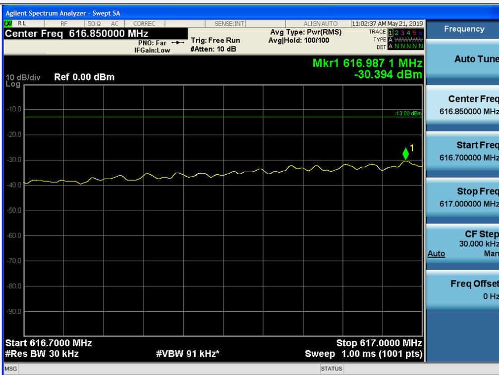
+3 dB above Out-of-band (single test signal) / 600 MHz Service / Downlink / LTE 5 MHz / Upper
