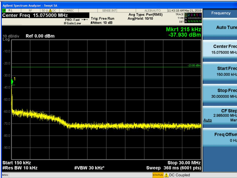
Spurious / 600 MHz Service / Downlink / LTE 10 MHz / Middle / 30 MHz ~ Low Edge - 10.1 MHz - 10.1 MHz
