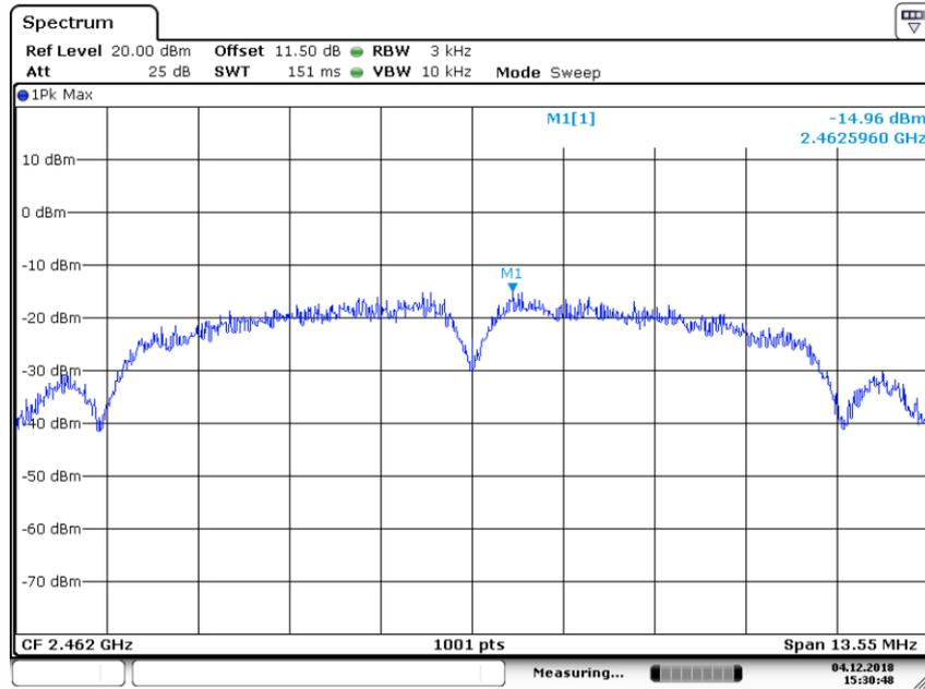
Test Model Power Spectral Density
