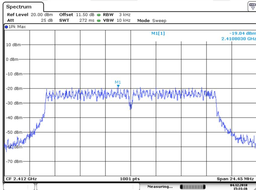
Test Model Power Spectral Density
