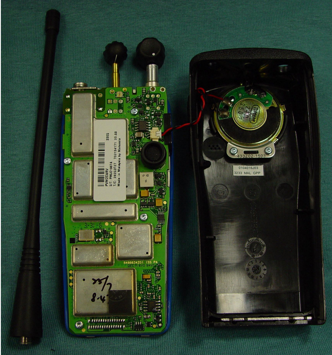
FRONT VIEW WITH CIRCUIT BOARD REMOVED FROM HOUSING (MATING SURFACES OF CIRCUIT BOARD AND HOUSING ARE SHOWN)
