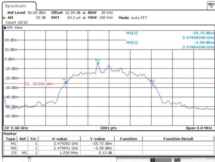
**99% OCCUPIED BANDWIDTH****DH1\_Ant1\_2402MHz**
