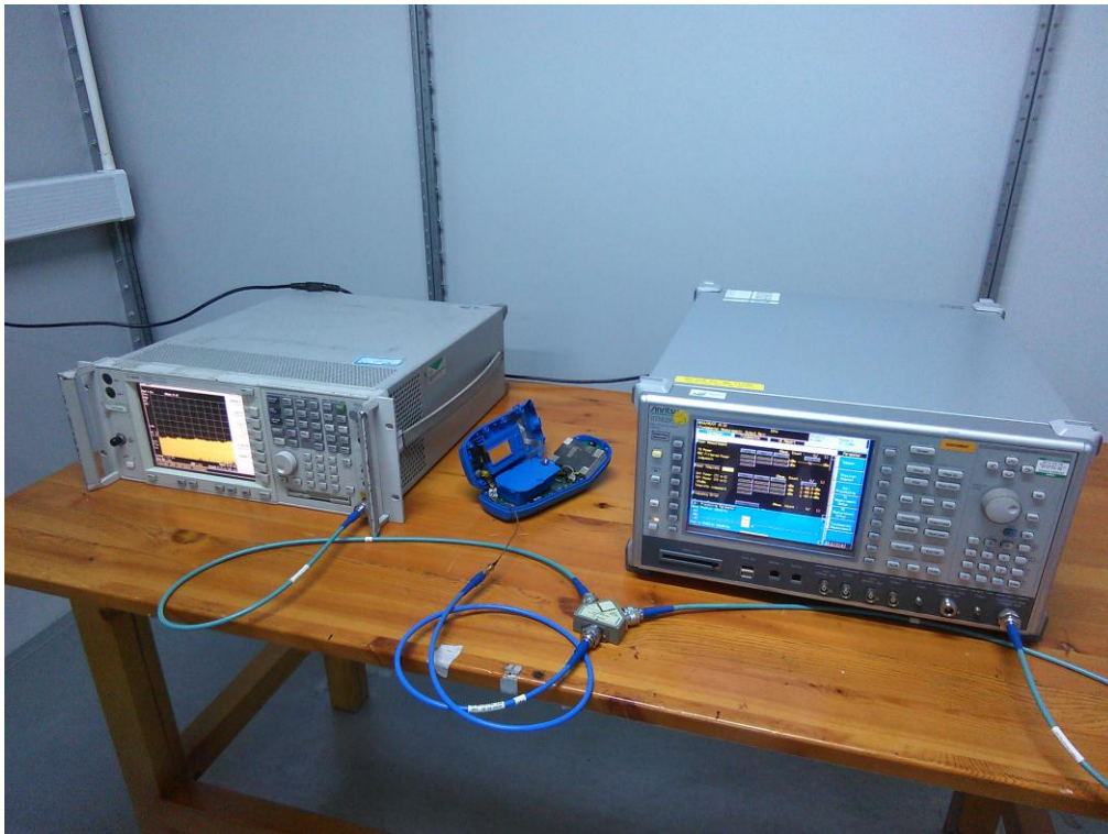
Photograph 1: Set-up for Conducted output power at Antenna Port
