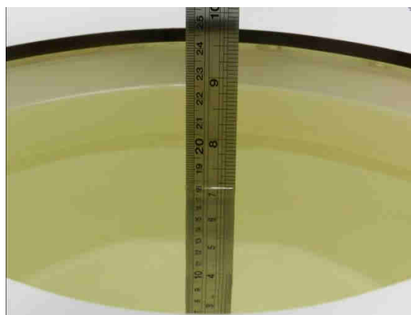
Fig 10.2 Photo of Liquid Height for Body SAR
