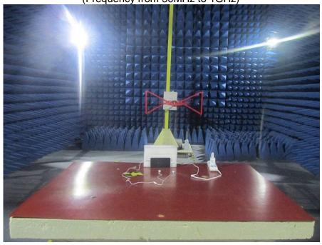
RADIATED EMISSION TEST (Frequency above 1GHz)
