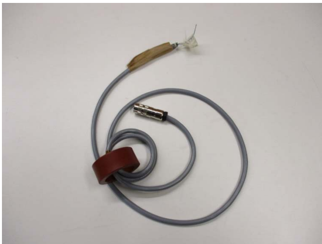
Photograph 2.3-3: Signal and supply cable with ferrite connected
