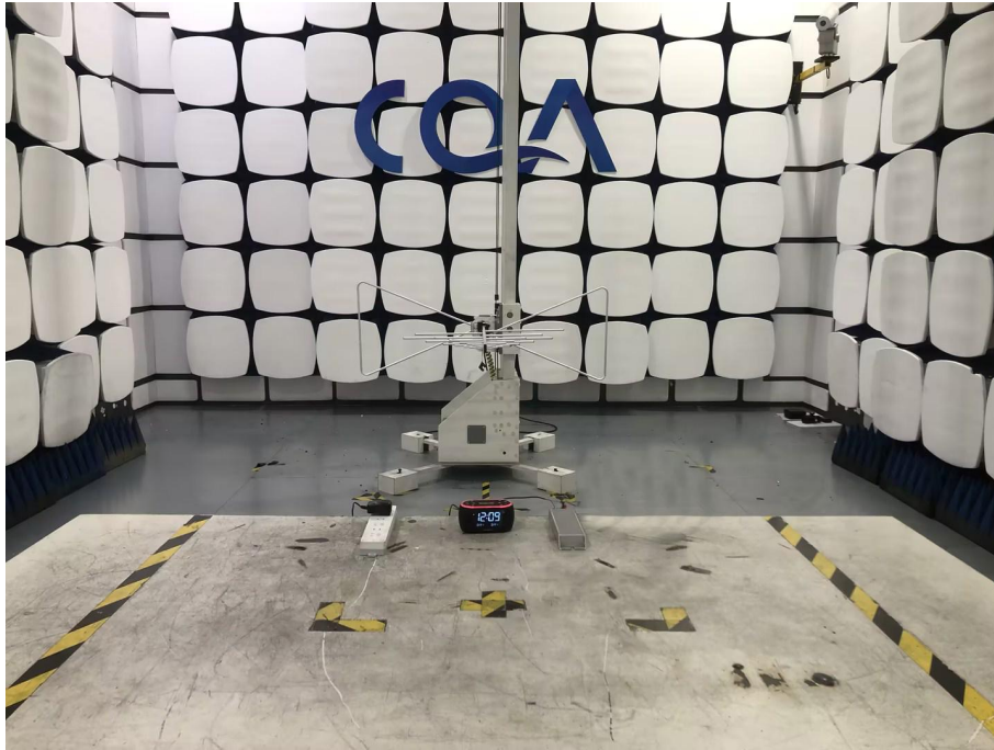
Radiated emission Test Setup (30MHz~1GHz)
