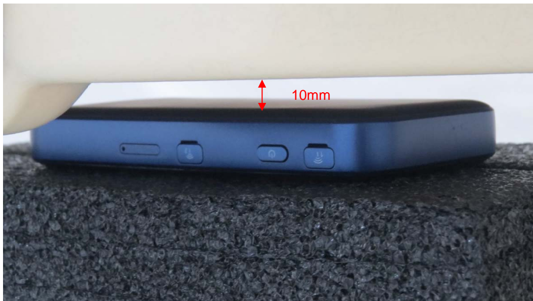
Picture 1: Back Side, the distance from handset to the bottom of the Phantom is 10mm
