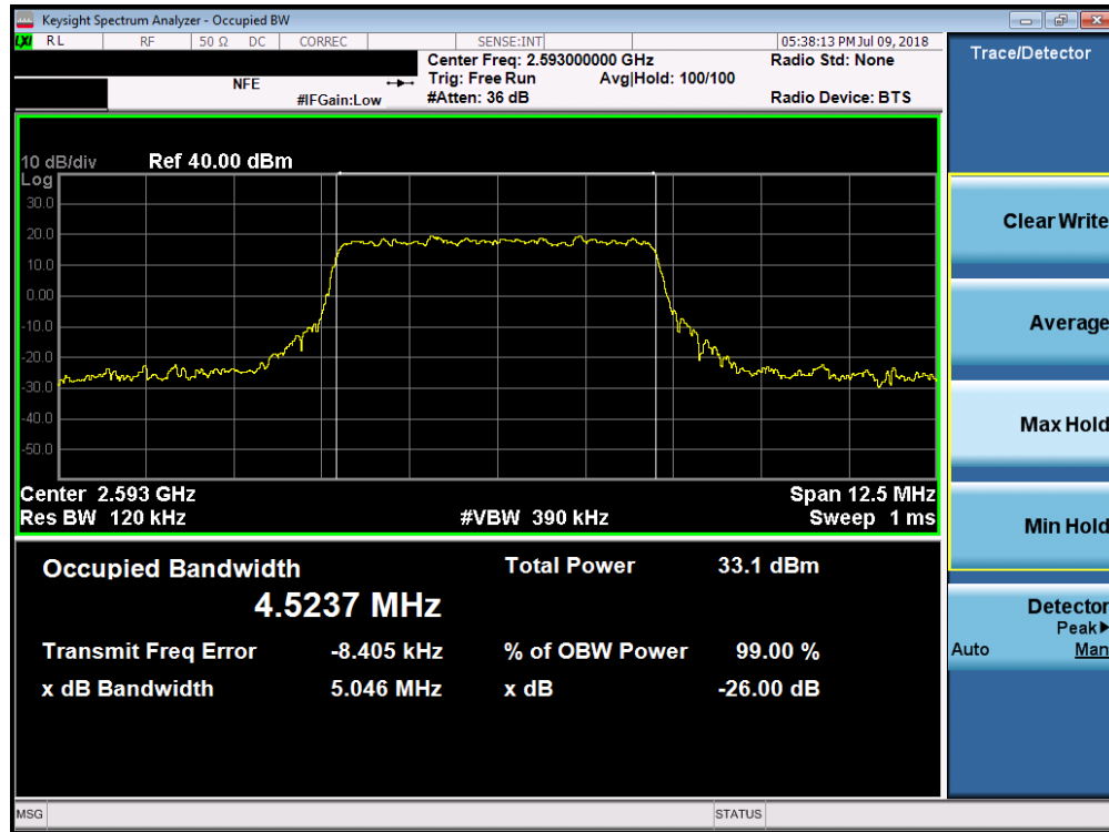
Plot 7-85. Occupied Bandwidth Plot (Band 41 - 5.0MHz QPSK - Full RB Configuration)
