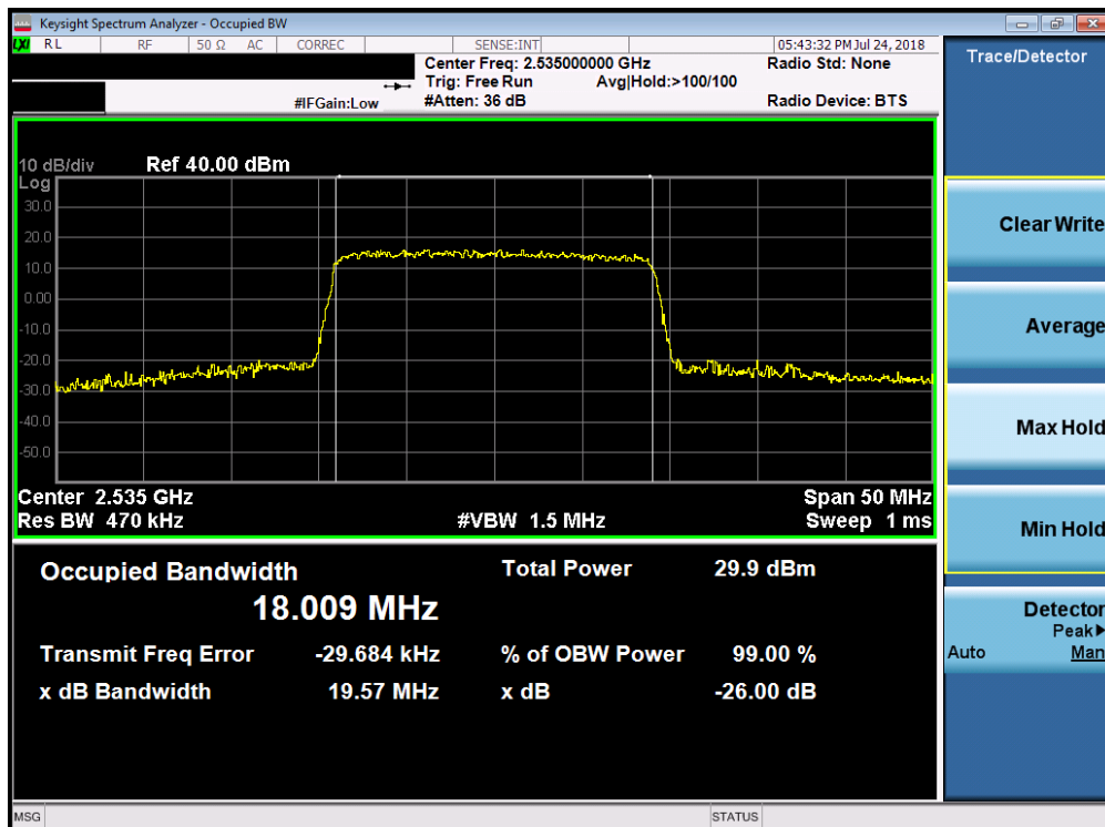
Plot 7-84. Occupied Bandwidth Plot (Band 7 - 20.0MHz 64-QAM - Full RB Configuration)
