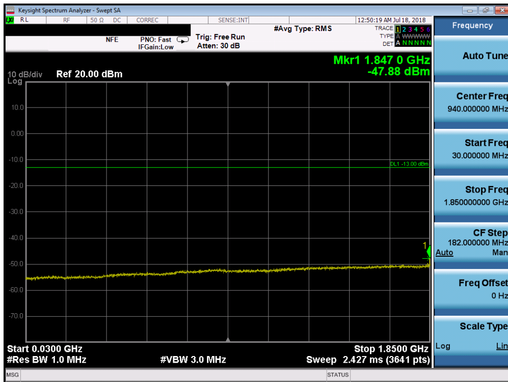
Plot 7-130. Conducted Spurious Plot (Band 25/2 - 20.0MHz QPSK - RB Size 1, RB Offset 0 - Mid Channel)
