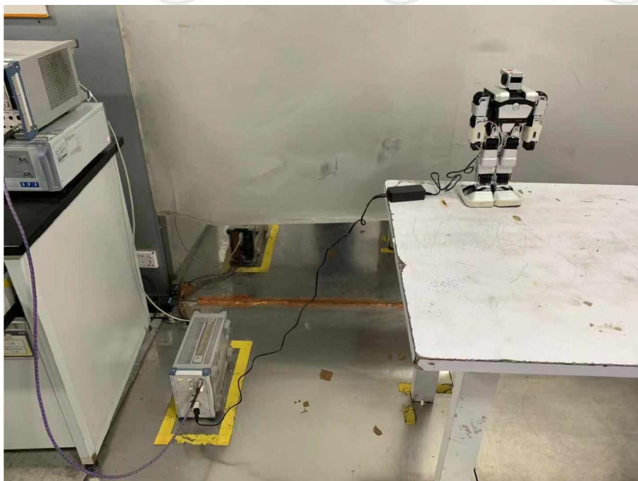
Conducted Emissions Test Setup
