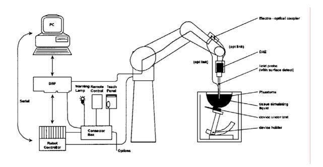
The DASY4 system for performing compliance tests consists of the following items:
