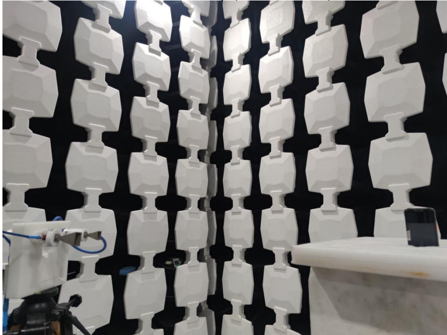
Description: Radiated Emission Test Setup (Above 18GHz)
