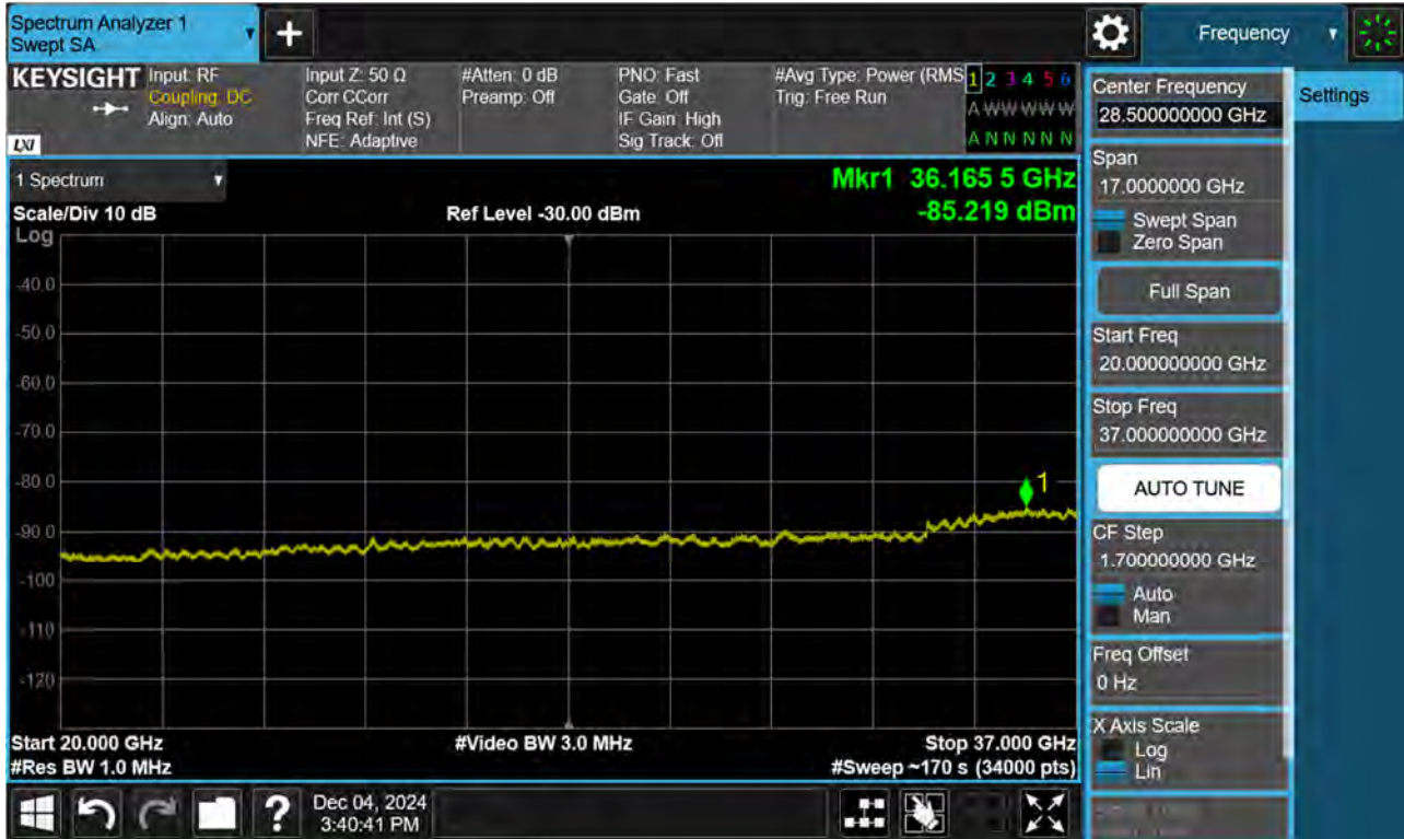
BAND 48. Conducted Spurious Plot 1 (15 MHz Ch.55315 QPSK RB 1, Offset 0)
