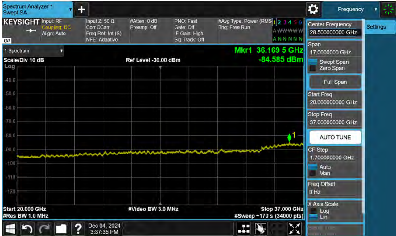
BAND 48. Conducted Spurious Plot 1 (10 MHz Ch. 56690 QPSK RB 1, Offset 0)
