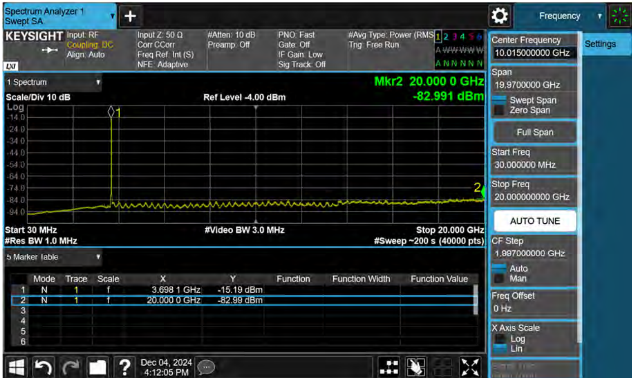
BAND 48. Conducted Spurious Plot 2 (5 MHz Ch. 56715 QPSK RB 1, Offset 0)
