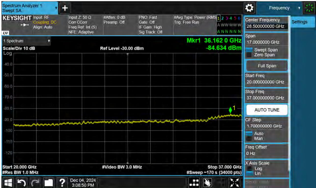
BAND 48. Conducted Spurious Plot 1 (5 MHz Ch.55265 QPSK RB 1, Offset 0)
