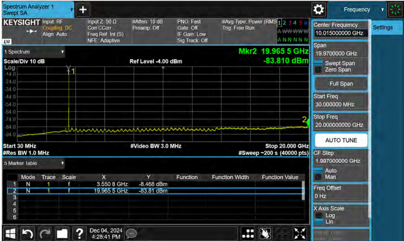
BAND 48. Conducted Spurious Plot 2 (15 MHz Ch. 55315 QPSK RB 1, Offset 0)
