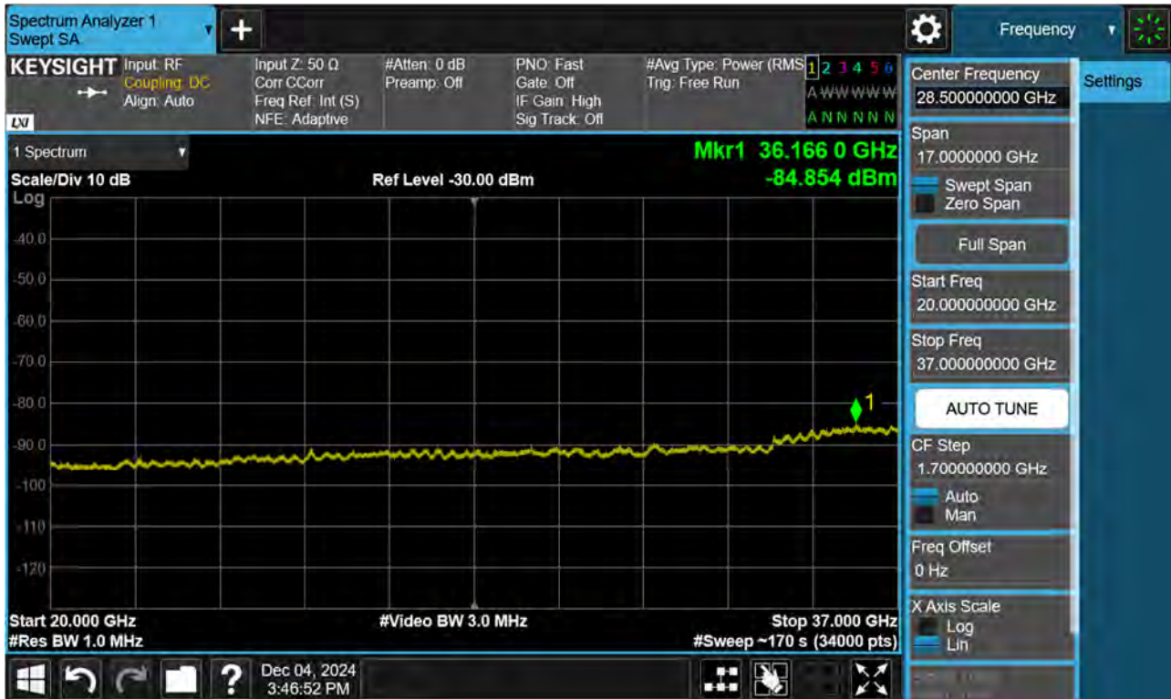
BAND 48. Conducted Spurious Plot 1 (15 MHz Ch.56665 QPSK RB 1, Offset 0)
