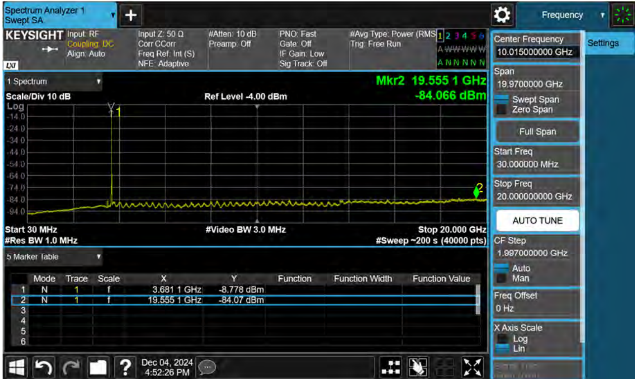
BAND 48. Conducted Spurious Plot 2 (20 MHz Ch. 56640 QPSK RB 1, Offset 0)
