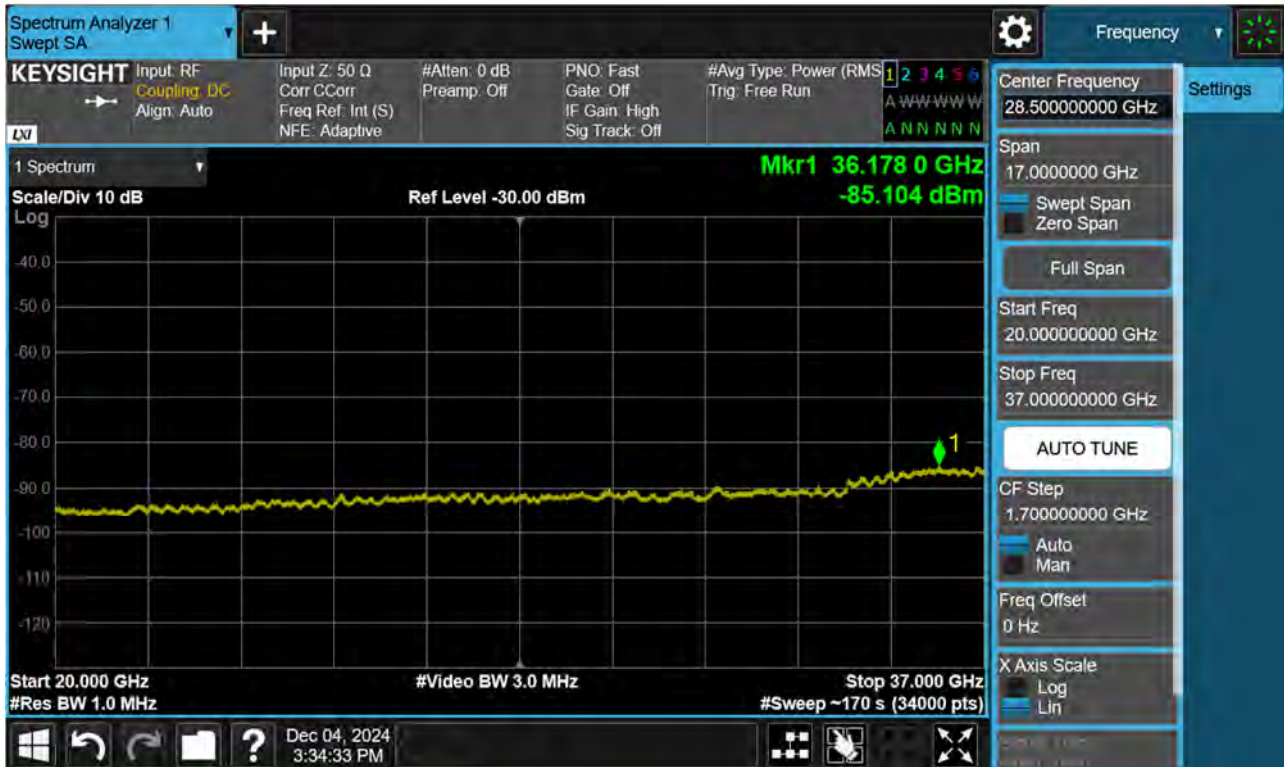
BAND 48. Conducted Spurious Plot 1 (10 MHz Ch.55990 QPSK RB 1, Offset 0)
