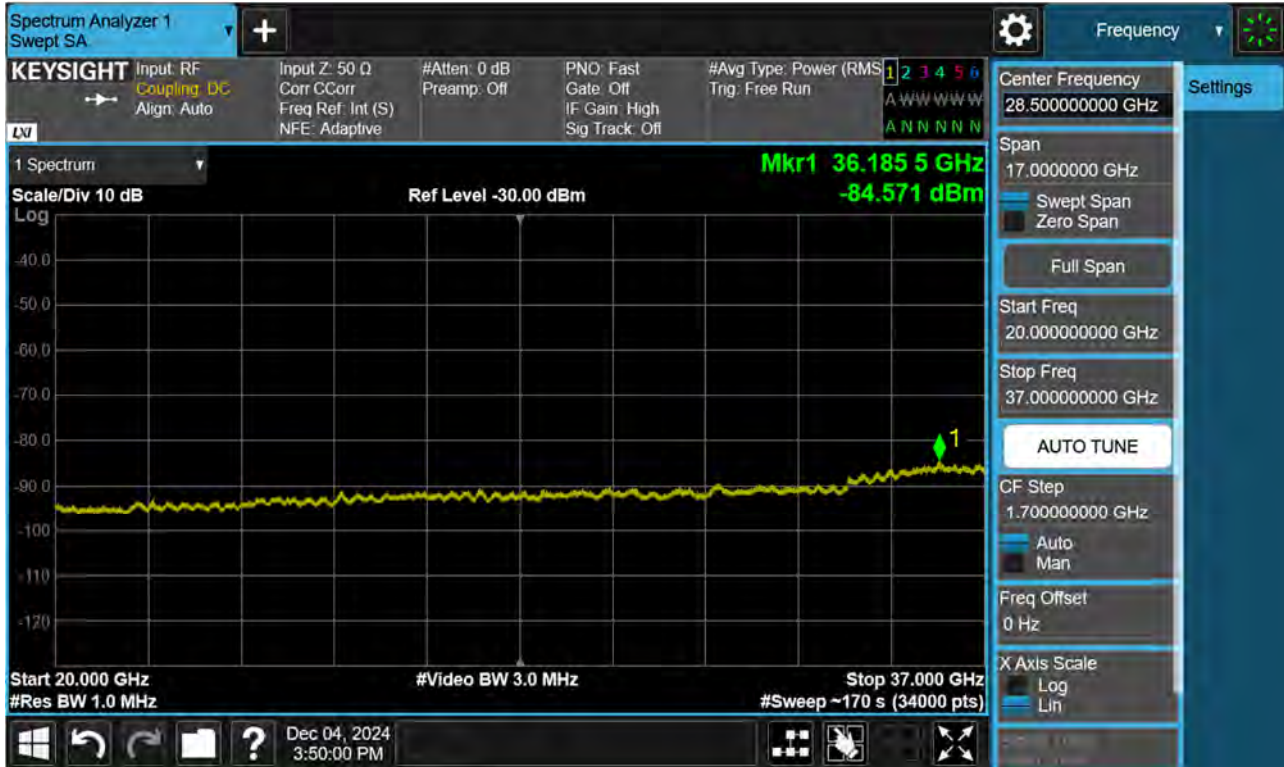
BAND 48. Conducted Spurious Plot 1 (20 MHz Ch.55340 QPSK RB 1, Offset 0)
