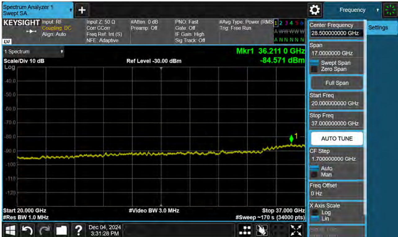
BAND 48. Conducted Spurious Plot 1 (10 MHz Ch.55290 QPSK RB 1, Offset 0)
