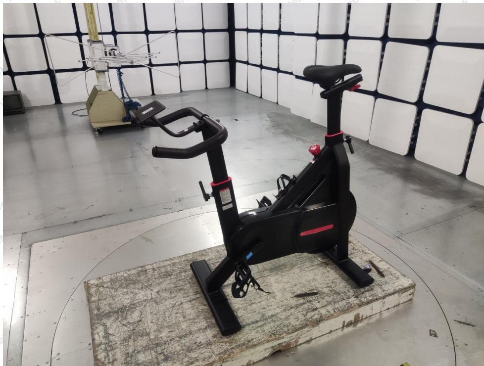
Photo of Radiation Emission Test
