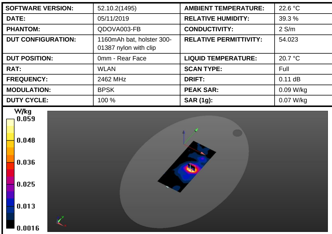
Figure 31: SAR Body Testing Results for the SC2028 at 2462 MHz.
