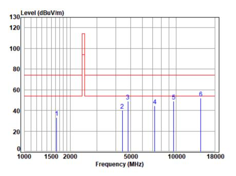
Site : chamber Condition: 3m VERTICAL : 01554AT Mode : 2410 TX RSE
