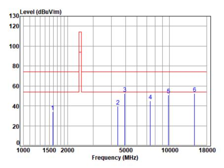
Site : chamber Condition: 3m VERTICAL : 01554AT Mode : 2470 TX RSE
