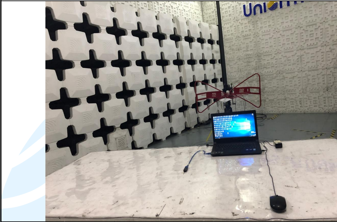
Radiated emission Test Setup (30 MHz~1 GHz)
