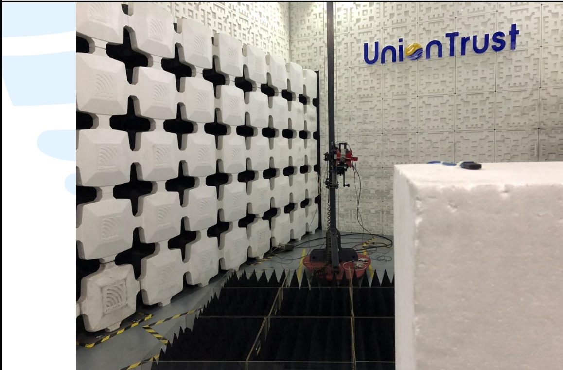
Radiated emission Test Setup (Above 1 GHz)
