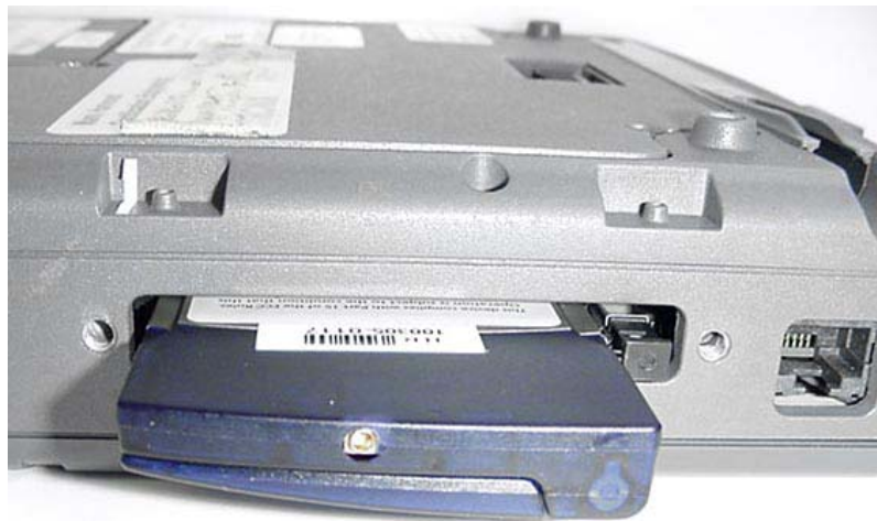
AirCard 580 installed in IX325 PCMCIA Slot (Broadband Hatch & Antenna Removed)
