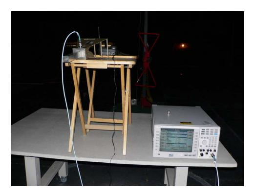
**TX Radiated Emission - Rear View**
