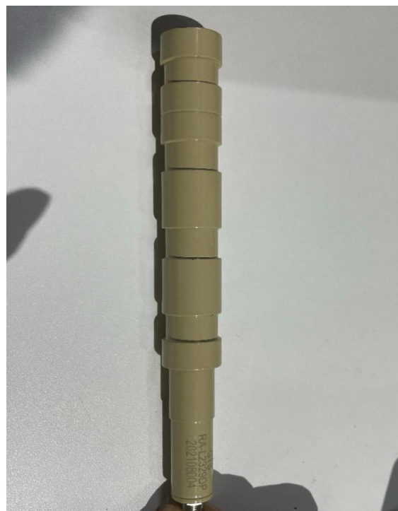
Fig 1 dipole model RA-L2329DP frequency 2300~2900 MHz
