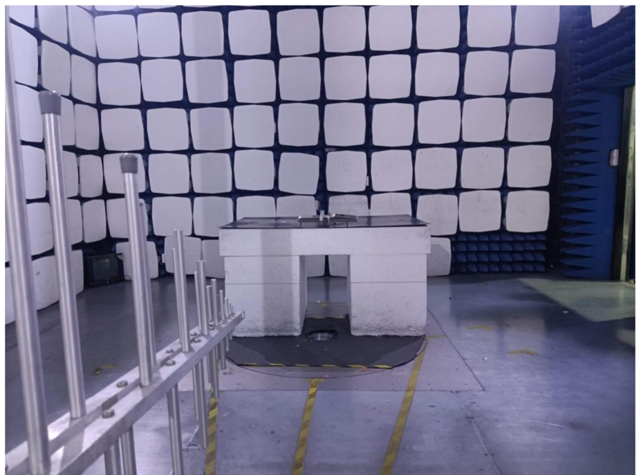
Radiation Emission Test Setup (30MHz to 1GHz)
