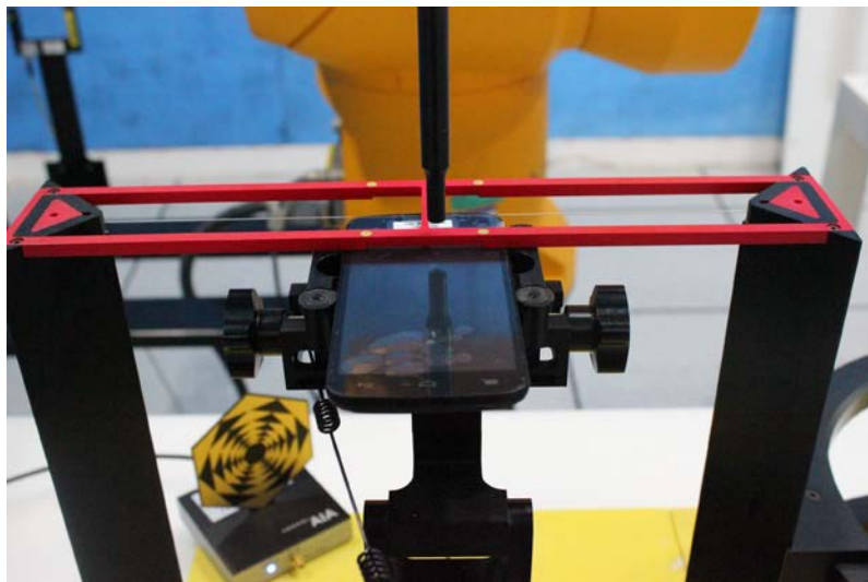
Picture 2: EUT Positioning for RF
