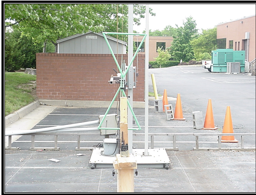
PHOTOGRAPH 2: RADIATED EMISSIONS TEST CONFIGURATION - FRONT VIEW
