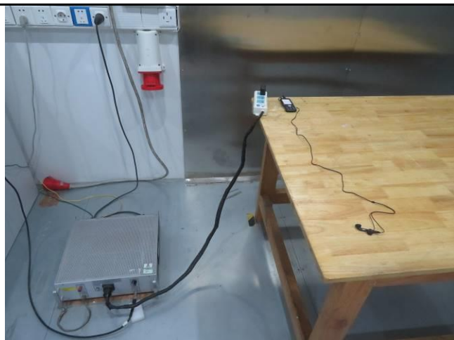
Conducted Emissions Test Setup Front View
