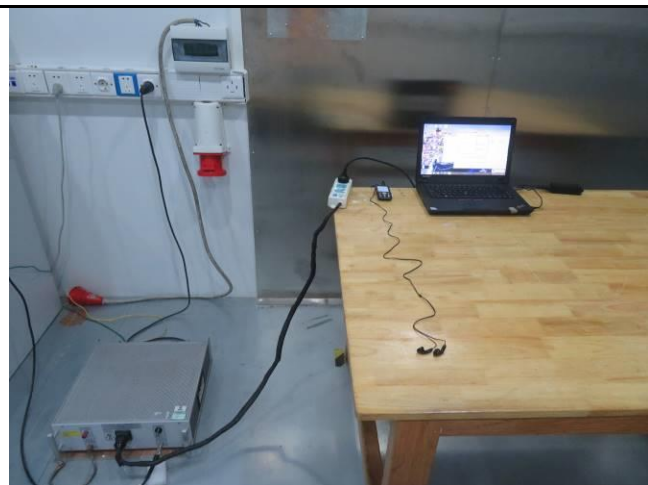
Conducted Emissions Test Setup – Front View
