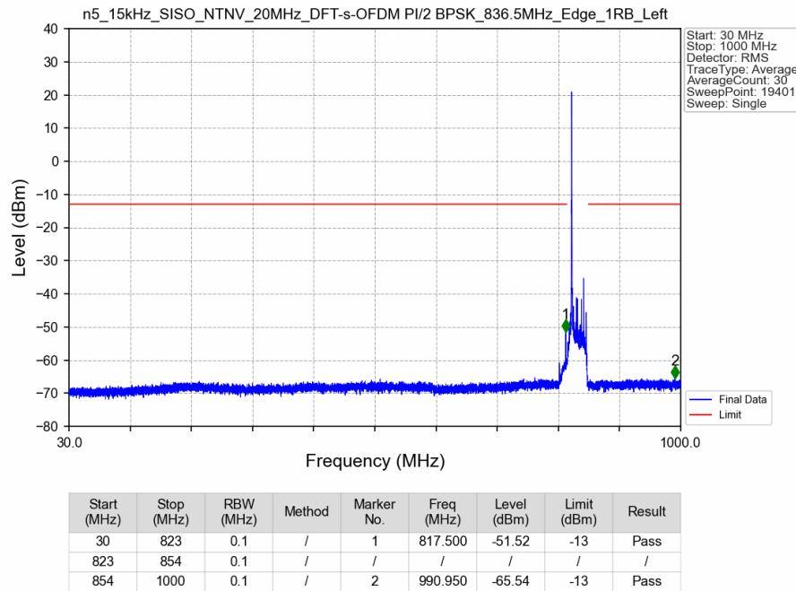
n5\_15kHz\_SISO\_NTNV\_20MHz\_DFT-s-OFDM PI/2 BPSK\_836.5MHz\_Edge\_1RB\_Left\_Ant0
