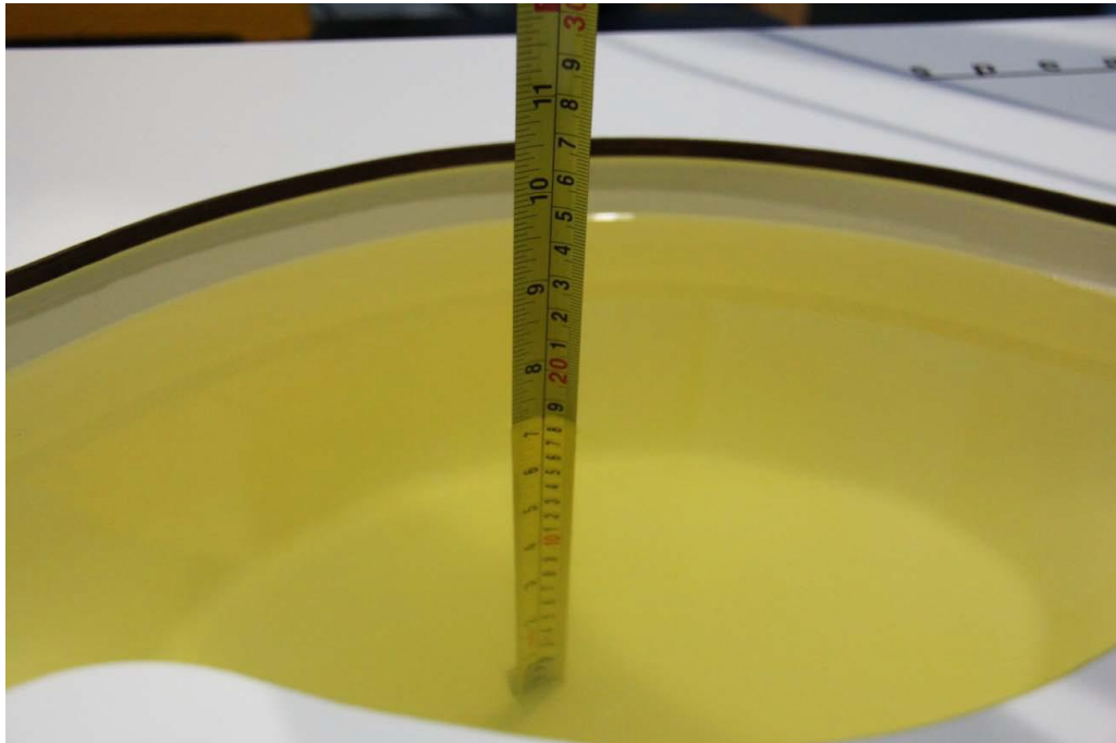
Picture 7-1: Liquid depth in the Flat Phantom(2450MHz)
