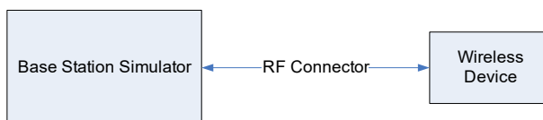
Figure 9-2 Power Measurement Setup
