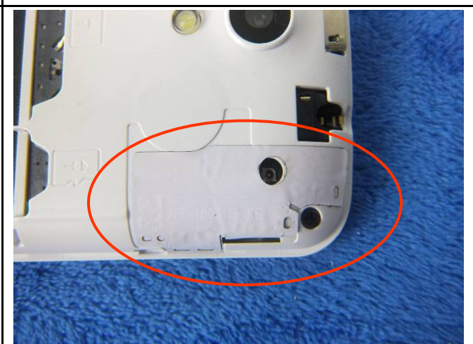
LTE - Antenna View
