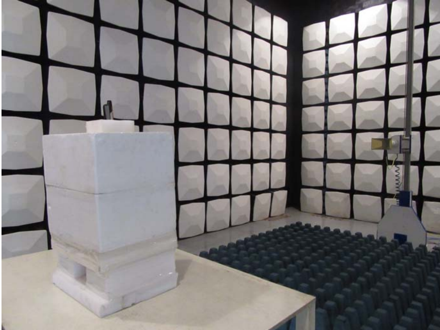
Radiated Emission View (Above 1GHz)
