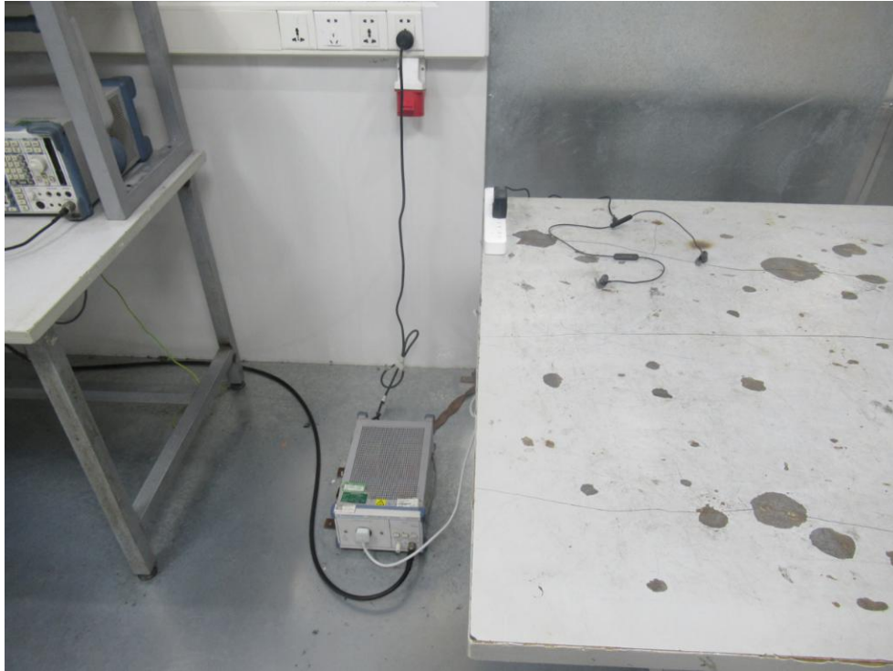
Photo of Conducted Emission Measurement
