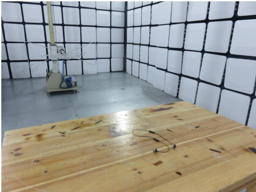
Photo of Radiation Emission Test
