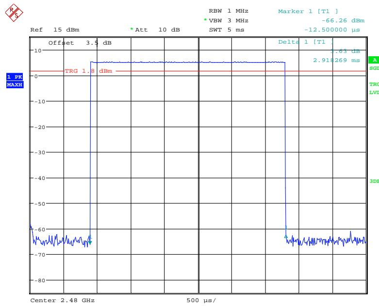
**EDR ( $\pi/4$ -DQPSK):****Pulse time, Low Channel, 2DH1**
