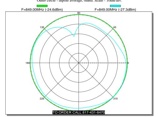
At 824MHz, the antenna gain is (-26.8) - (-23.3) = -3.3 dBdAt 849MHz, the antenna gain is (-27.3) - (-24.6) = -2.7 dBd
