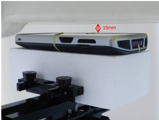
Front, Test Separation 15 mm
