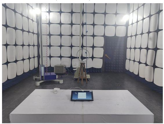
3. Radiated emission (9KHz-30MHz)
