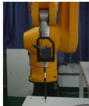
Picture C.3 E-field Probe
