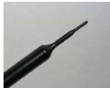
Picture C.2 Near-field Probe
