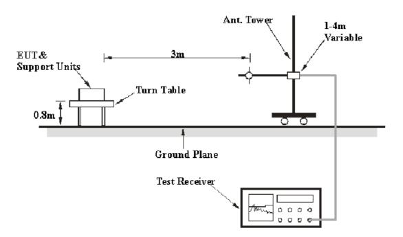
The radiated emission tests were performed in the 3-meter Chamber B using the setup accordance with the ANSI C63.4-2003. The specification used was the FCC 15.109(a) limits.
