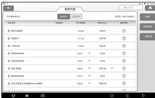
On the software upgrade page, click [One-click Upgrade] to start downloading. After the download is complete, the system will automatically install the software.
