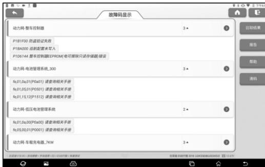
Systems with fault codes are displayed on the screen in red font with the specific number of fault codes. The system without faults (green) is displayed as "Normal".
