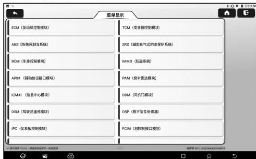
Select the electronic control system to be tested. The function selection page is
