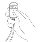
1. Press and hold the MI or MII button for two seconds to store station. When the MI or MII icon blinks, release the button.
